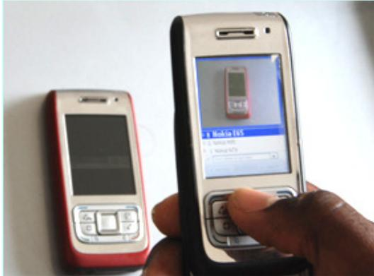
**Figure 1: Point&Find, a vision-based mobile interface. The object is recognized in real-time, candidate results are ranked and listed below the view finder window.**
