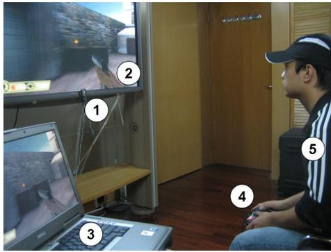
**Figure 9. Test setup of Bullet Time, showing camera (1), plasma display (2), computer with game (3), joystick (4) and player (5).**
