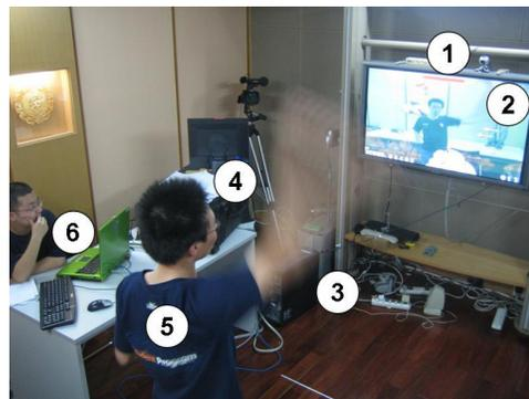
Figure 8. Test setup of Diver, showing camera (1), plasma display (2), computer with game (3), video taping system (4), player (5) and instructor (6).
