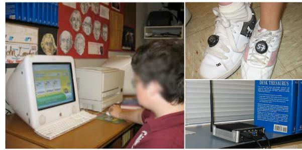
**Figure 1.** A student viewing school status on the AHPC website (left); Pedometers clipped on the shoes (upper right); Wireless station that collects data from pedometers within range (lower right).
